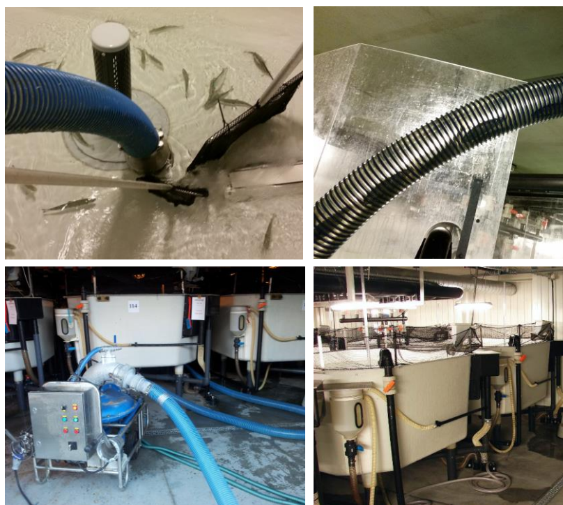
Figure 2: Equipment and setup for pumping of fish. Before pumping with a Heathro Vaki pump, the water level was lowered with 1/3 the original level, in order to facilitate pumping
